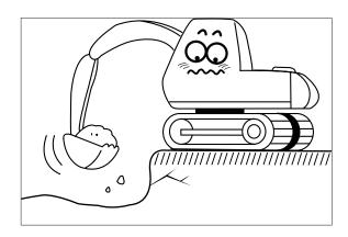
Operate for the lifting work considering the capacity of machine, weight and width of the load. Be careful not to lift exceeding the machine capacity as it can be the cause of machine damage and safety accident.
